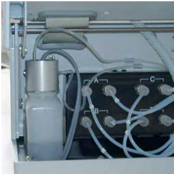
Re-insert the rear-seal wash solution reservoir.
